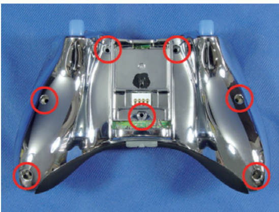
12. Close the controller bottom, put on the 7 screws then cover the battery pack back to the place.
